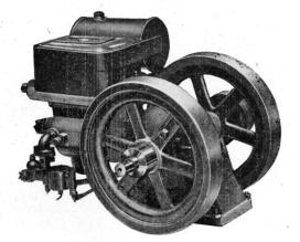
The ARLINGTON X. L. ENGINE is the natural evolution and combination of the single cylinder, horizontal valve-in-the-head, hopper cooled, enclosed crank case type with throttling governor.
